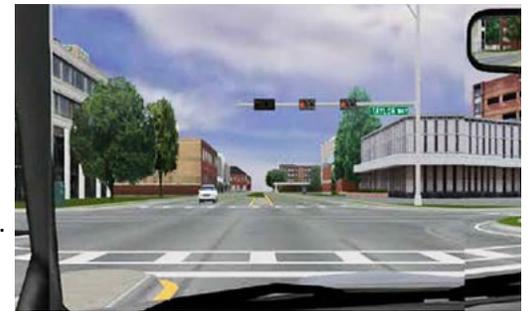
*Simulator view of an intersection with a flashing yellow arrow controlling the left turn lane.*
